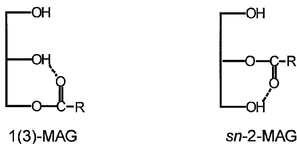
FIG. 6. Structures showing possible internal hydrogen bonding in the two classes of MAG, leading to equivalent polarity (Ref. 14). See Figure 1 for abbreviation.
